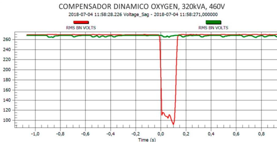
*The red line represents the input voltage where the voltage drops down up to 91.8 volts and the green line represents the same phase but compensated by OXYGEN.*
